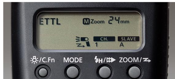
When the 430EXII is set to this option it will function as a remote slave flash unit controlled by a master flash unit such as a Canon 580EX II or ST-E2 Speedlite Transmitter. The master and slave(s) must be set to the same communication channel. Slaves set to a different channel than the master will not trigger. You can select from four channels, numbered 1 – 4.
