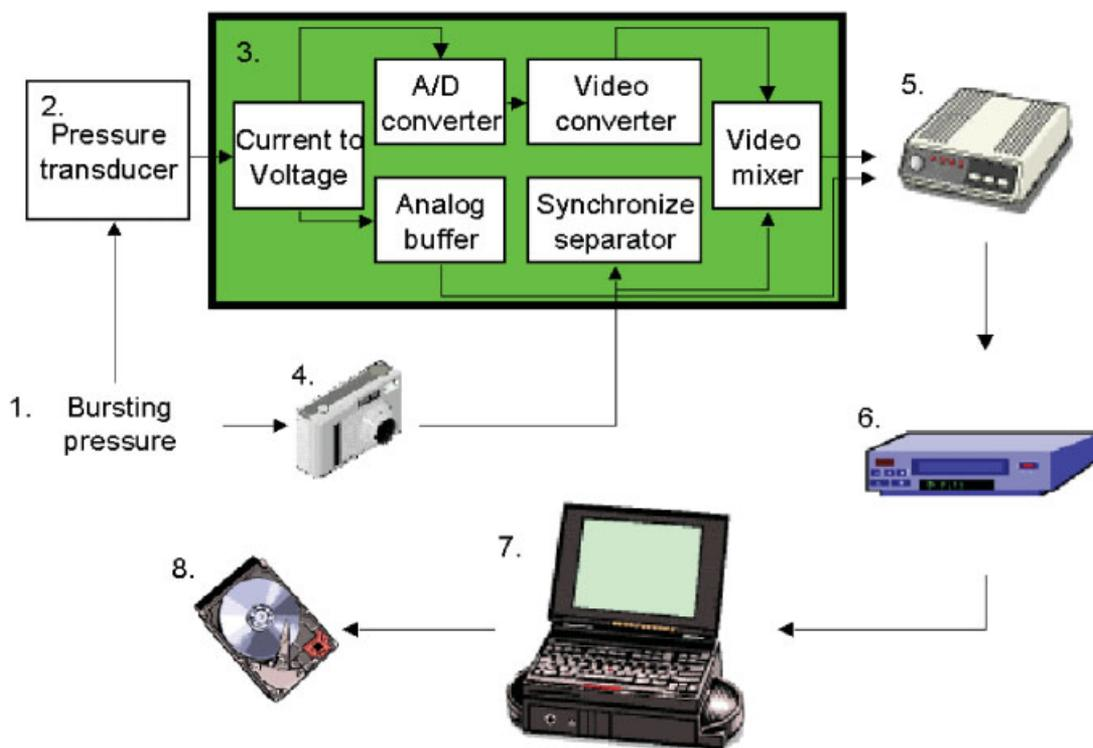
Fig. 1. A schedule representing the model to determine the bursting pressure of the treated right iliac artery as illustrated in the photograph (1). The 2F sheet is linked to a pressure manometer and a pressure transducer coupled (2) to a converter module matrix (3). The analog voltage signal evoked by the pressure is converted to digits in the video screen. These digits are integrated in the display of the bursting pressure
