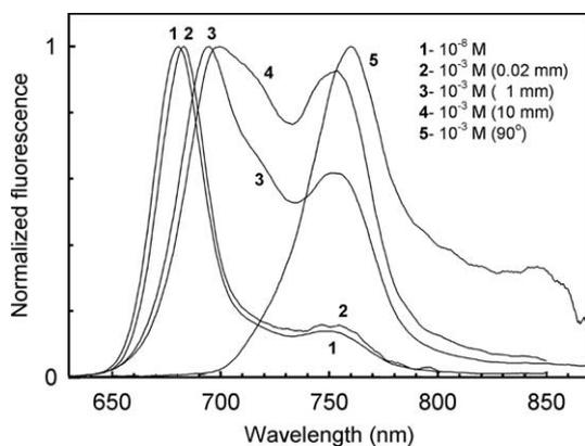
Fig. 2. Fluorescence emission spectra of AlPcS<sub>4</sub> at a low concentration ( $10^{-8}$  M, curve 1, standard cuvette holder) and a high concentration ( $10^{-3}$  M, curves 2–4, measured with the fibre-optic probe, curve 5 – standard cuvette holder).
