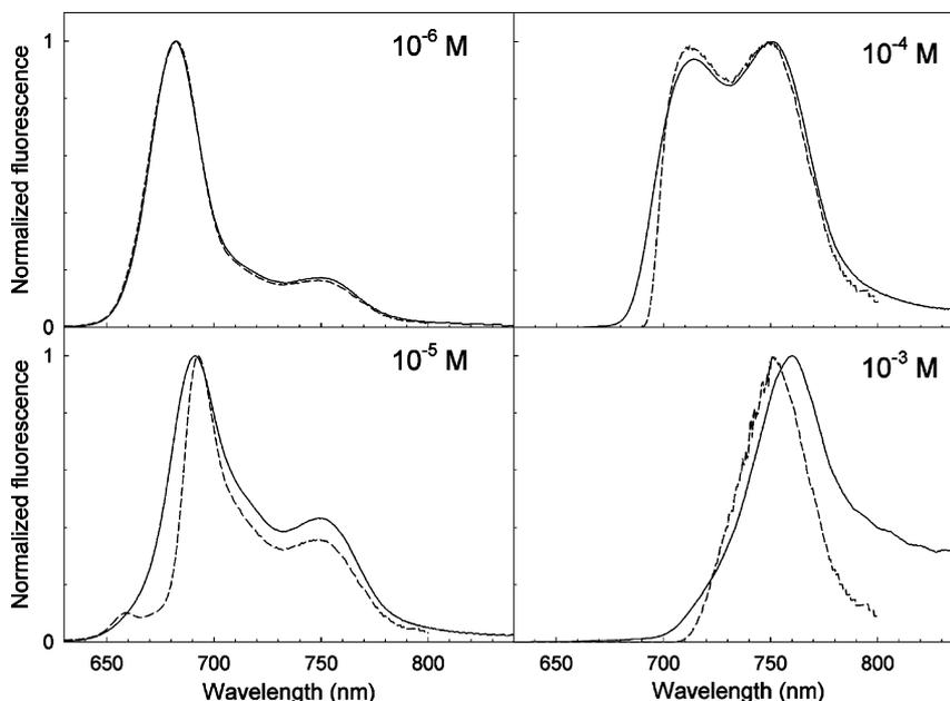
Fig. 3. Measured (solid lines, from Fig. 1(b)) and calculated (dashed lines, from Eq. (1)) fluorescence spectra of AlPcS<sub>4</sub> at various concentrations taking into account the inner-filter effect. The geometrical constant used in the calculations is  $k(10^{-6}$  M) = 0.1,  $k(10^{-5}$  M) = 1.3,  $k(10^{-4}$  M) = 15 and  $k(10^{-3}$  M) = 200.
