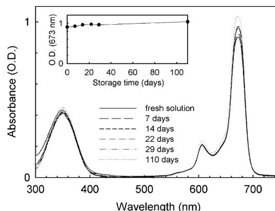
Fig. 4. Stability of AlPcS<sub>4</sub> solution ( $10^{-5}$  M) stored at room temperature (20–25 °C). Absorption spectra were measured in a quartz cuvette (pathlength 5 mm). Inset shows a peak value at 673 nm.
